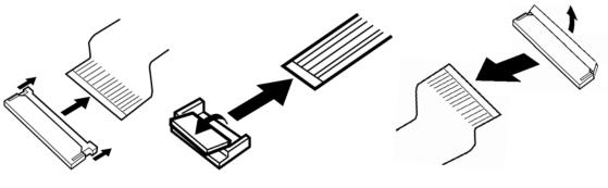
Pressure plate connector Spring connector
